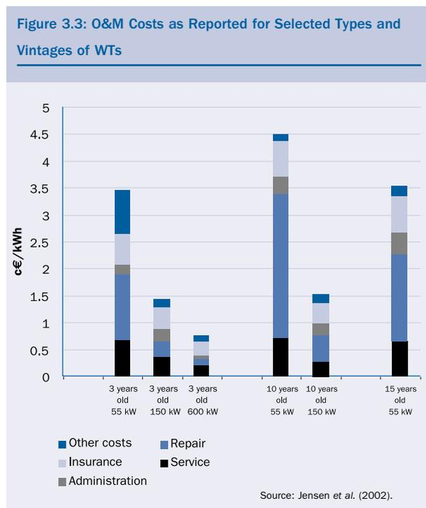
Figure 3.3 clearly shows the trend towards lower O&M costs for new and larger machines. Thus, for a three-year-old turbine, O&M costs have decreased from approximately 3.5 c€/kWh for the old 55 kW machine to less than 1 c€/kWh for the newer 600 kW. The figures for the 150 kW WT are almost at the same level as the O&M costs identified in the three countries mentioned above.
