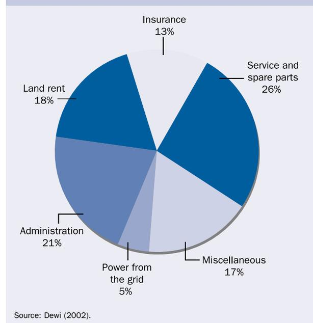
Figure 3.2: O&amp;M Costs Reported for Selected Sizes and Types of Wind Turbines
